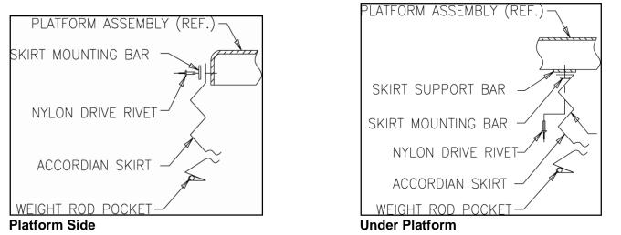
4. Install weight rods into weight rod pockets at bottom of accordion skirt. Install spring tempered wire rods into pocket of black convolutions.
