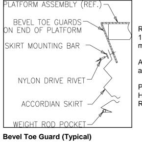
Raise one side of skirt along with a skirt-mounting bar (1/8" x 1") to side of bevel toe guard. When possible, center skirt-mounting collar and skirt-mounting bar (1/8" x1") on platform.
