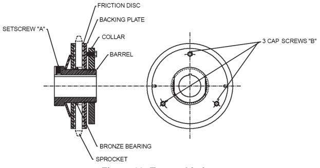
Figure 18: Torque Limiter
