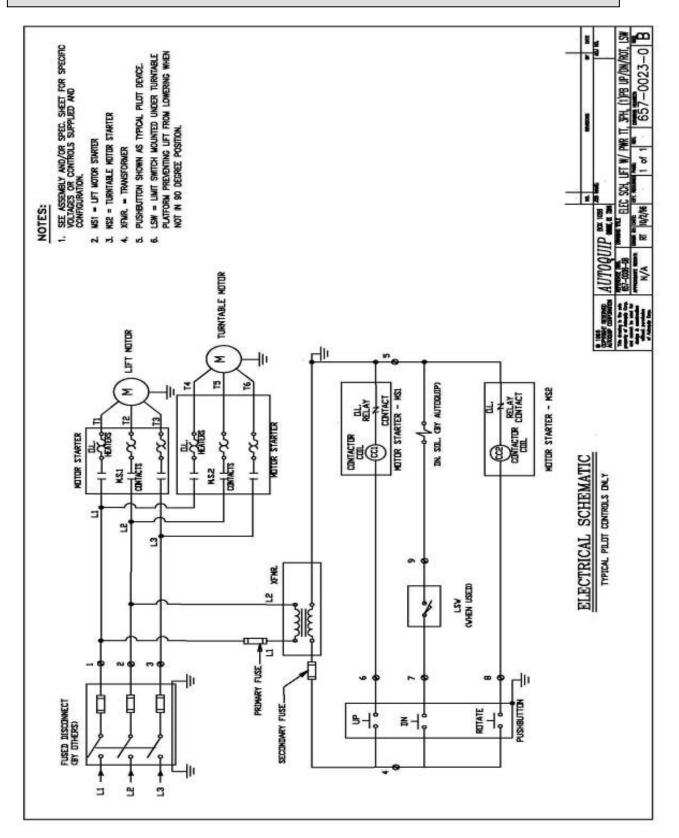
Figure 13: SRP Electrical Schematic <u>208-230-460V/3PHASE</u>, Single Direction Rotation w/ Lift DOWN LIMIT SWITCH – UP/DOWN & Rotate
