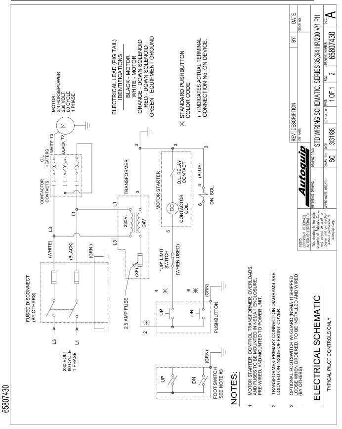
Figure 20: STE-30/45 Electric Schematic; 230V / 1Ph
