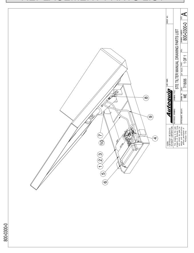
Figure 28: STE Tilter Parts Diagram
