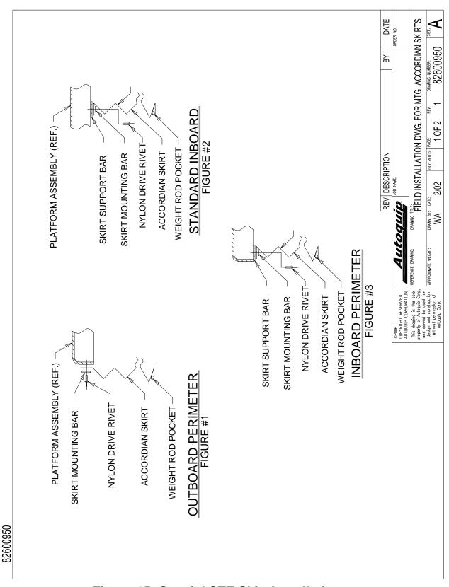
Figure 15: Special STE Skirt Installation
