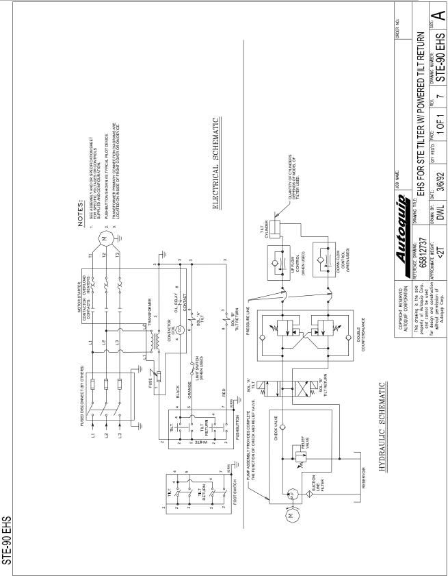
Figure 22: STE-90 Electrical & Hydraulic Schematic:208-230-460V/3Ph
