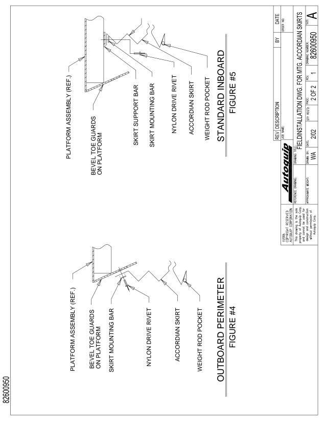
Figure 16: STE Skirt Installation for Bevel Toe Guards
