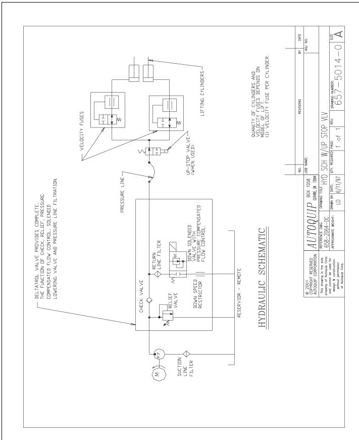
Hydraulic Schematic; Heavy Duty Power Unit
