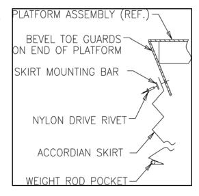
4. Install weight rods into weight rod pockets at bottom of accordion skirt. Install spring tempered wire rods into pocket of black convolutions.
