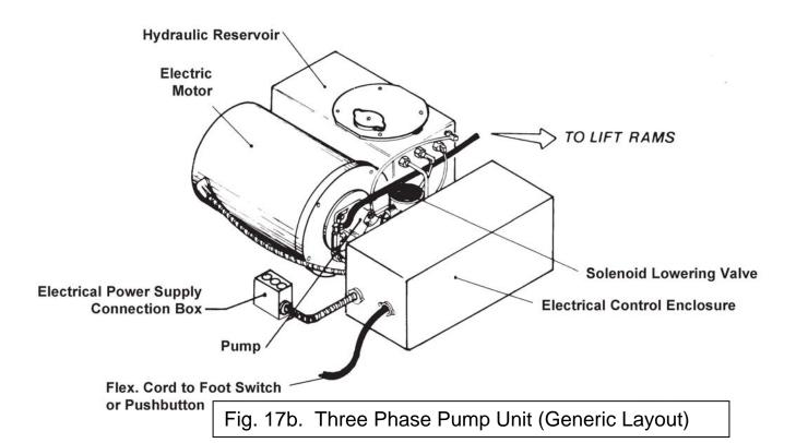
Figure 17. Parts Idenification – Pump Unit
