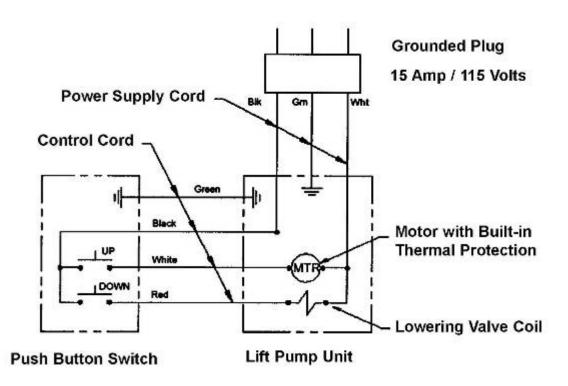
Figure 15: Push Button Wiring Details – 115VAC/Single Phase
