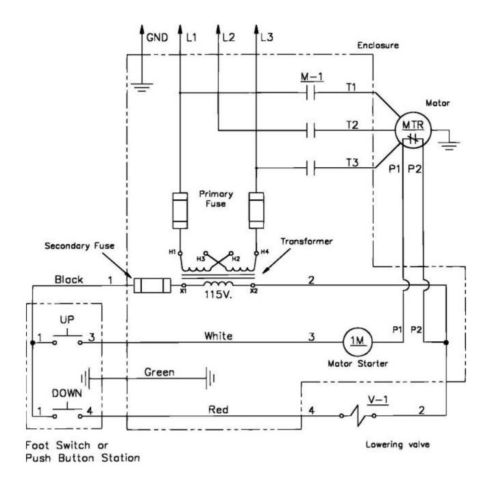
Figure 16. Generic Electrical Schematic 208-230-460V – 3phase
