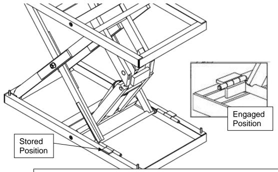
Fig.10a. Maintenance Device – (2) Maintenance Locks
