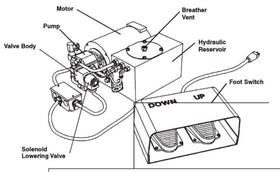
Fig. 17a. Single Phase Pump Unit (Generic Layout)
