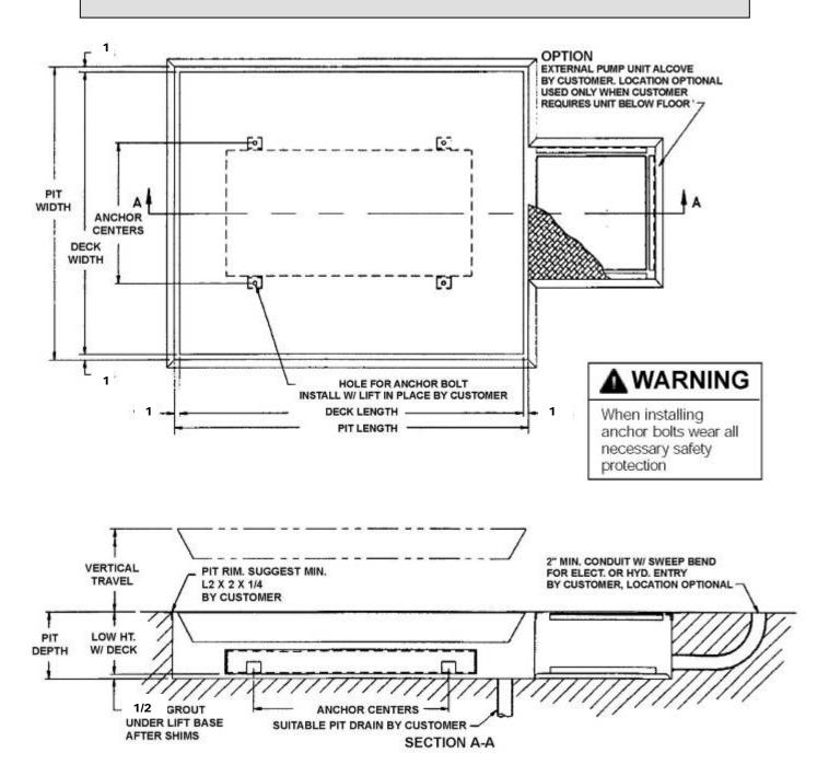
Figure 11: Typical Pit Detail
