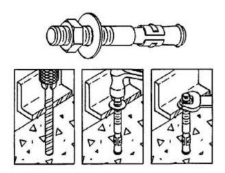
Figure 12: Anchor Detail
