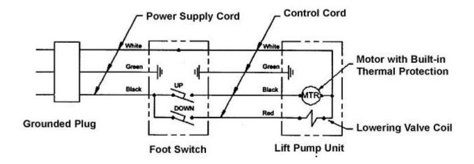
Figure 14: Foot Switch Wiring Details – 115VAC/Single Phase
