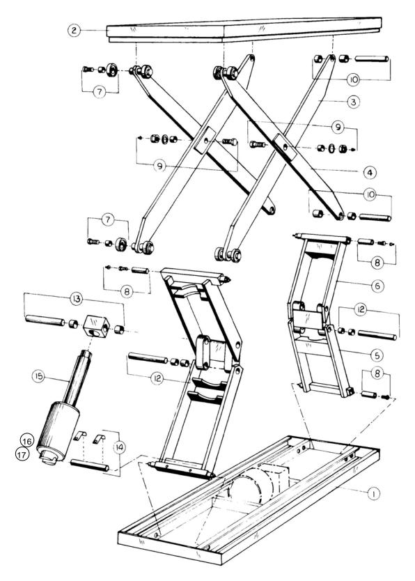
Figure 19. Replacement Parts Diagram – Double Arm Lift
