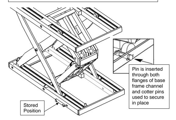
Fig. 10b. Maintenance Devices – (2) Roller Base Pins
