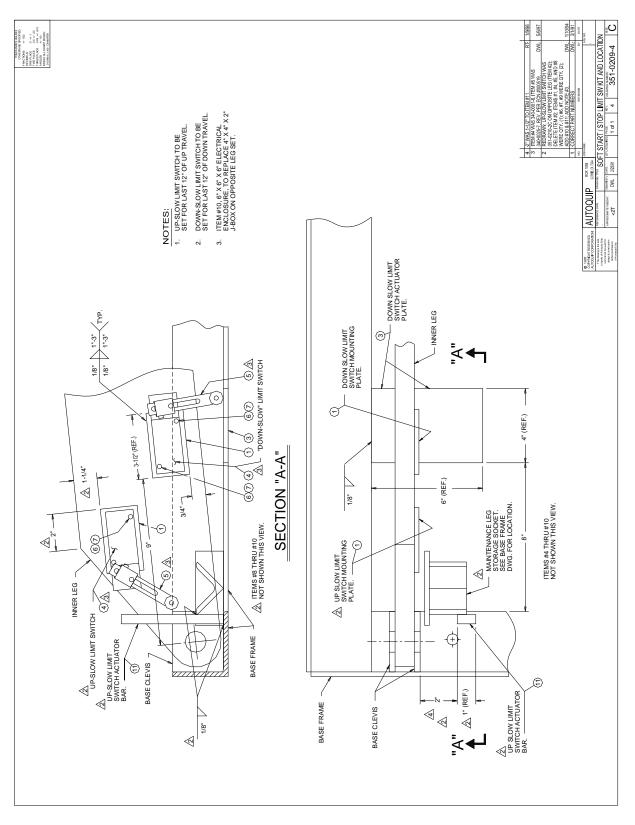
Figure 19 – Limit Switch Location – Soft Start/Soft Stop
