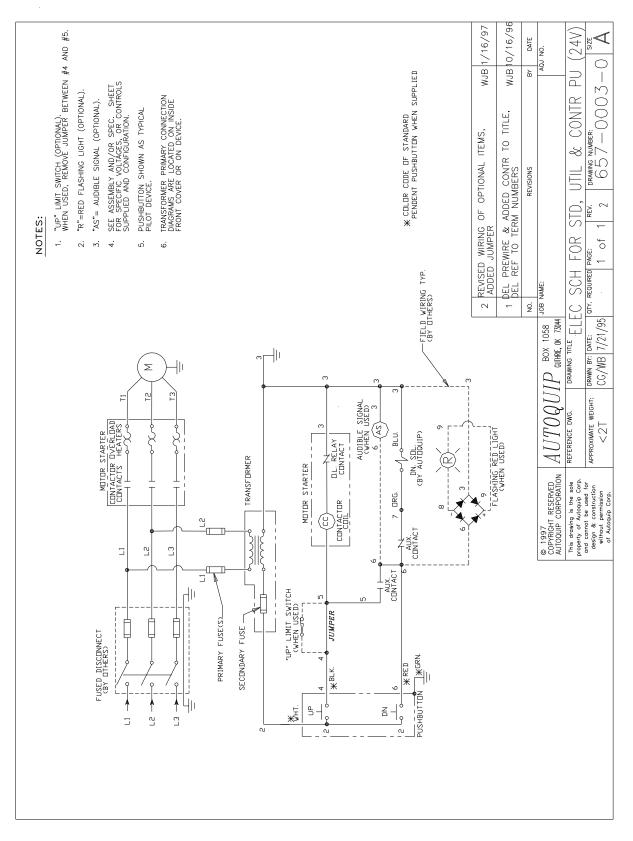
Figure 14 Electrical Schematic – 208-230-460 Volt Three Phase
